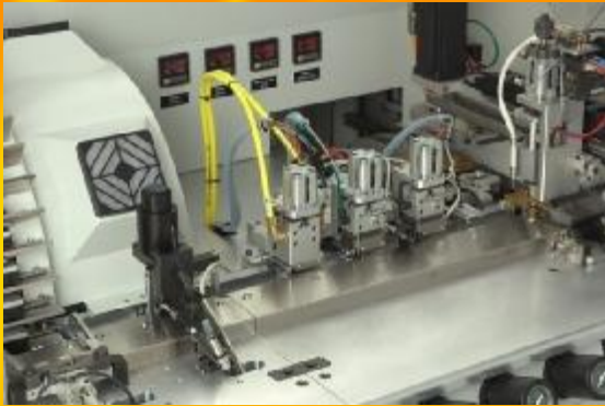
Chip embedding module with pressers heads
